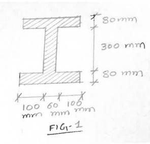
(II) Calculate & draw shear stress diagram for a simply supported beam as shown in fig-3. cross section of a beam is shown in Fig-2.
